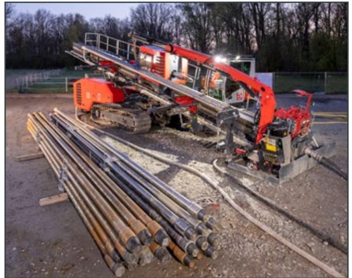
Figure 1: HDD80-E –STREICHER's fully-electric driven HDD rig
