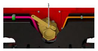
Fig. 4-6: Drain cock on the container
