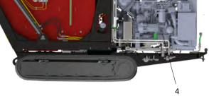
Fig. 6-1: BOE drain valves
