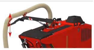
Lower suction arm slightly and (2) place clamp into appropriate latching (3) cam.
