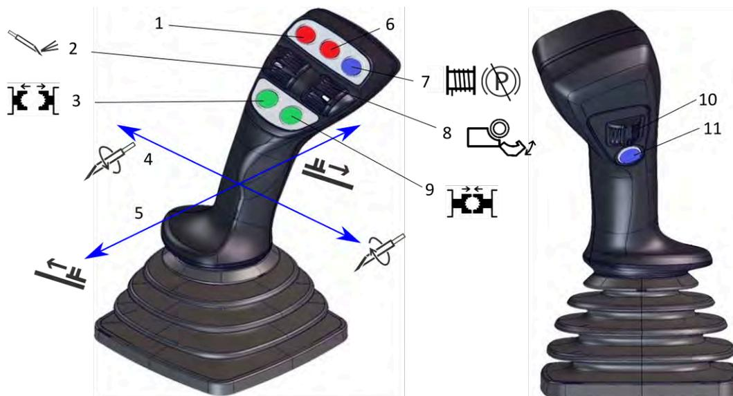
Abb. 5-6: Linker Joystick
