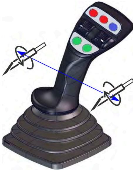
Abb. 7-30: Linker Joystick - Rotation
