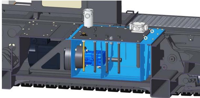
Abb. 4-16: Hydraulikaggregat
