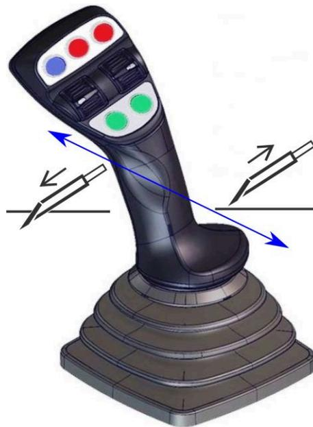
Abb. 7-26: Linker Joystick - Rotation
